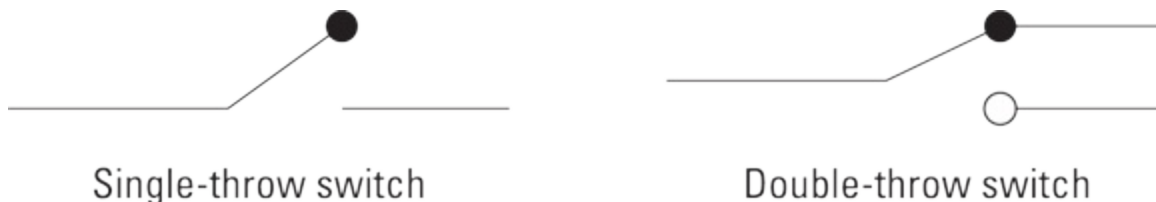
FIGURE 15-1: Two circuit symbols representing a switch.
