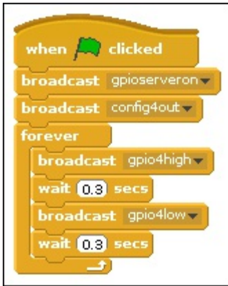
FIGURE 16-7: Scratch program to blink the LED.
