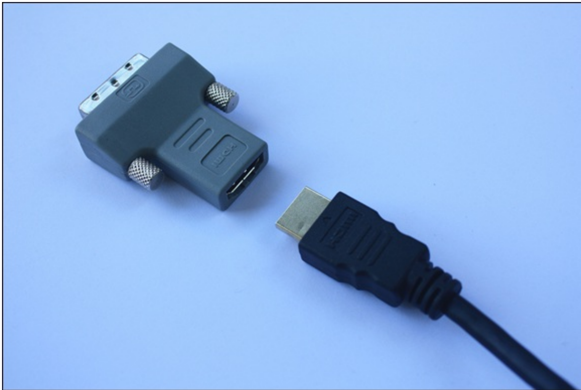
FIGURE 3-9: How the HDMI cable is inserted into the DVI converter.
