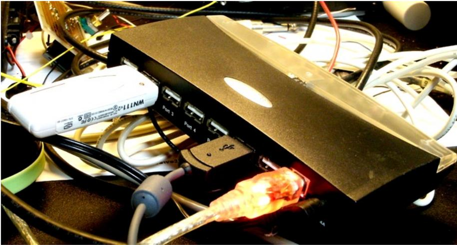
*Figure 8-2. A powered USB hub*
