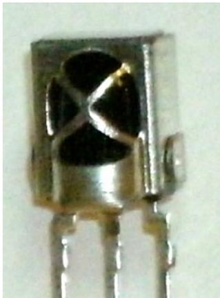
**Figure 26-1.** The VS1838B PIN photodiode
