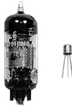
FIGURE 12-32 The Vacuum Tube vs. the Transistor
